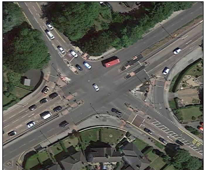
MOVA 8 can switch datasets by an input which was a key factor in allowing this junction to perform. MOVA 8 has the flexibility to change conditioning through the dataset which means there is greater control during the day to day optimisation process. The 6MRR code can manage the right turn movements effectively given the large variability both time of day and day to day.
